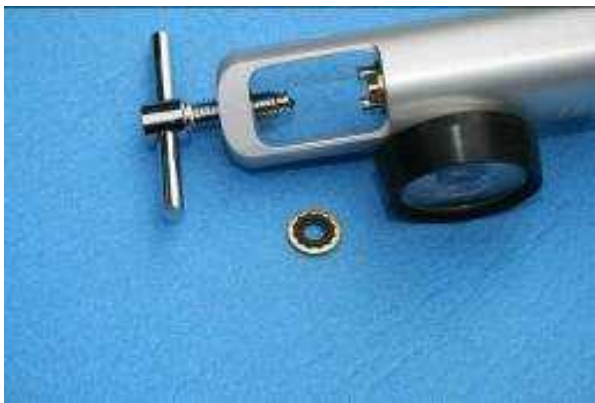
Verify condition of the regulator and washer.
