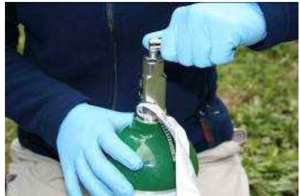
Open tank to expel any dust that may be in the system.
